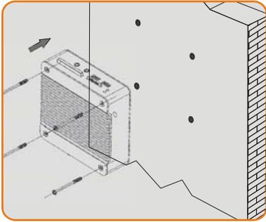
2: The following diagram shown machine of screw holes will be installed behind the display.
