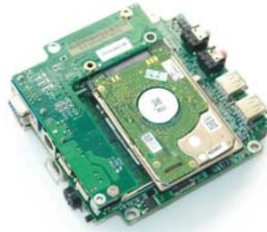
5: Install the finished expansion board into chassis and fix HDD with the drive bays.
