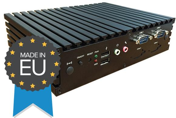
Fanless design, high efficiency and low power consumption make **TECHBOX X200** a perfect device for projects where long trouble-free operation is essential.
