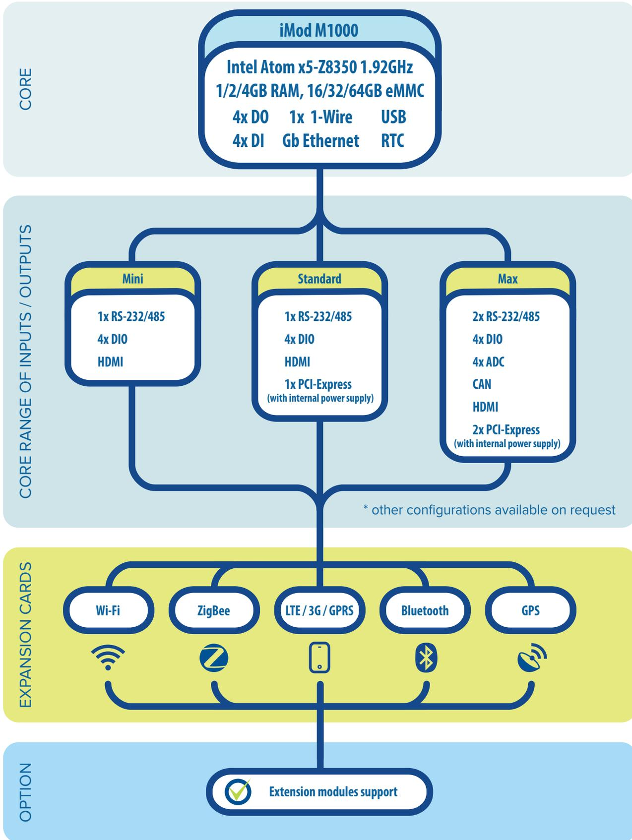
The **NPE M1000** device allows use of up to 3 expansion modules, increasing its capabilities with additional I/Os, providing support for additional modems and wireless communication modules, and adding new features such as accelerometer and opto-isolation.
